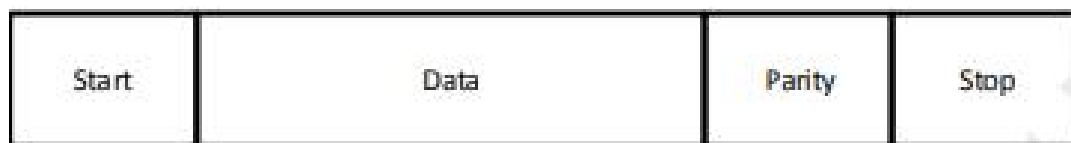
Figure 6-12. UART Data Frame
