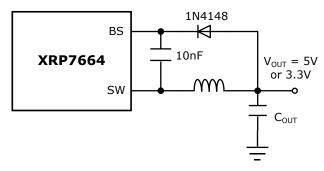
Fig. 17: Optional External Bootstrap Diode where  $V_{OUT} = 5V$  or 3.3V
