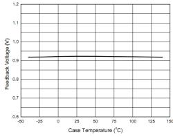
Fig. 7: Feedback voltage versus case temperature
