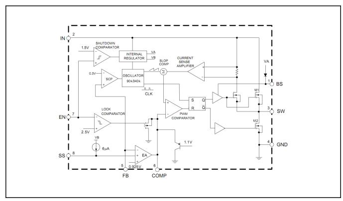
Fig. 2: XRP7664 Block Diagram
