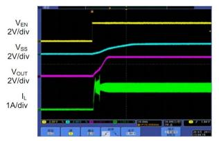
Fig. 12: Enable turn on  $(R_{LOAD}=1.65\Omega)$ Base Time 10ms/div
