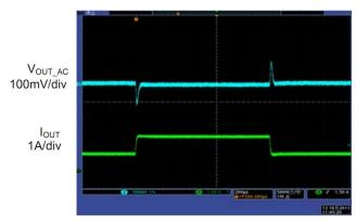
Fig. 11: Load transient ( $I_{OUT}$ =1A to 2A) Base Time 200 $\mu$ s/div
