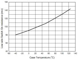
Fig. 6: R<sub>DSONL</sub> versus case temperature
