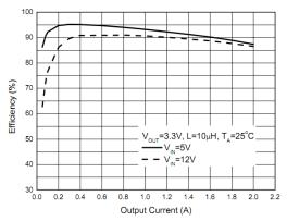
Fig. 4: Efficiency versus output current
