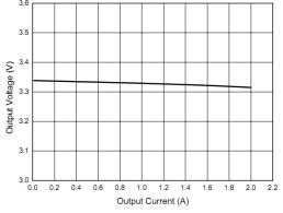
Fig. 9: Output voltage versus output current
