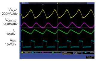
Fig. 10: Output voltage ripple,  $I_{OUT}$ =2A Base Time 2 $\mu$ s/div
