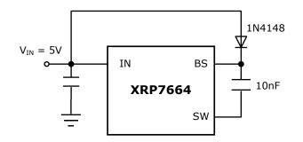
Fig. 16: Optional External Bootstrap Diode V<sub>IN</sub>=5V Fixed
