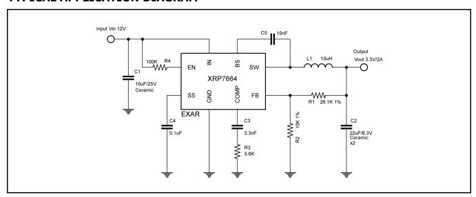
Fig. 1: XRP7664 Application Diagram
