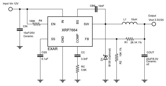
Fig. 18: XRP7664 Typical Application Diagram - 12V to 3.3V Conversion
