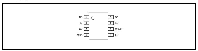
Fig. 3: XRP7664 Pin Assignment (SOIC-8)
