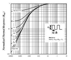
Fig 10. Effective Transient Thermal Impedance
