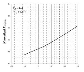
Fig 4. Normalized On-Resistance v.s. Junction Temperature
