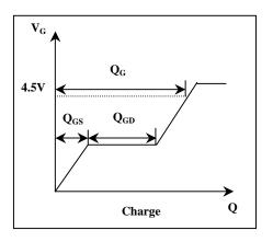
Fig 12. Gate Charge Waveform
