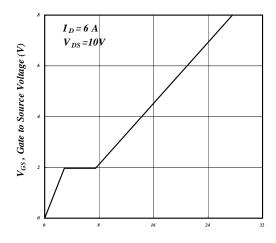
Fig 7. Gate Charge Characteristics
