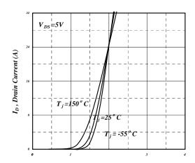
Fig 11. Transfer Characteristics
