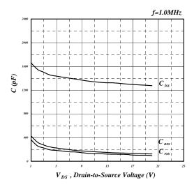
Fig 8. Typical Capacitance Characteristics
