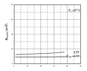
Fig 15. Typ. Drain-Source on State Resistance
