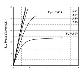
Fig 2. Typical Output Characteristics
