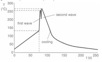
Total immersion exposure time for Sn/Ni terminations is 30s at a wave temperature of 260°C. Note that for multiple soldering operations, including the rework, the soldering time is cumulative.
