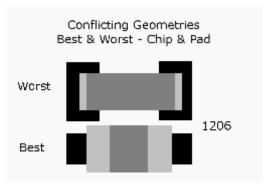
Reducing the pad/ land size can reduce the level of stress exerted onto the capacitor by approximately 50%.
