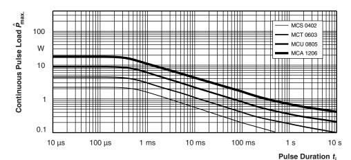
Maximum pulse load, continuous pulses; applicable if  $\bar{P} \leq P\left(\mathcal{S}_{amb}\right)$  and  $\hat{U} \leq \hat{U}_{max}$ ; for permissible resistance change equivalent to 8000 h operation in standard operation mode
