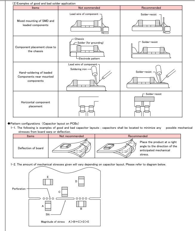
1–3. When PCB is split, the amount of mechanical stress on the capacitors can vary according to the method used. The following methods are listed in order from least stressful to most stressful: push-back, slit, V-grooving, and perforation. Thus, please consider the PCB, split methods as well as chip location.
