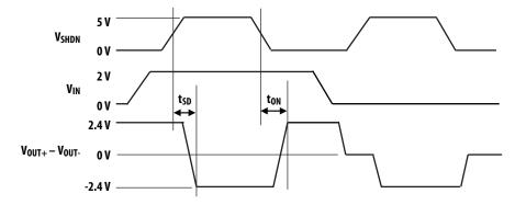
Figure 27: Propagation Delay Diagram
