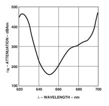
Figure 1. Typical POF attenuation vs. wavelength.
