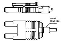
The duplex latching connector is designed for rugged applications requiring greater retention force than the nonlatching duplex connector. When inserting the duplex latching connector into a module, the connector latch mechanism should be aligned with the top surface of the dual combination of horizontal or vertical Versatile Link components. The duplex latching connector is available in gray (HFBR-4516Z).
