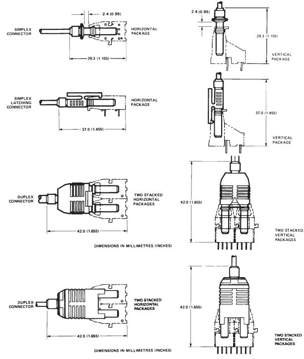
Bulkhead Feedthrough or Panel Mounting for HFBR-4501Z/4511Z Simplex Connectors
