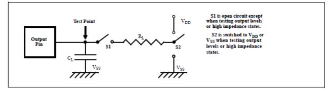
Figure 11 - Output Test Load
