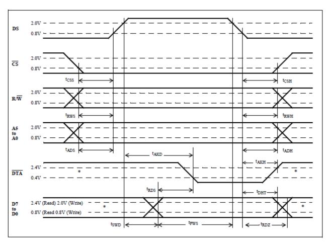
Figure 17 - Processor Bus
