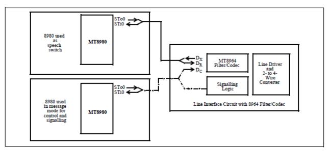
Figure 7 - Example of Typical Interface between 8980s and 8964s for Simple Digital Switching System
