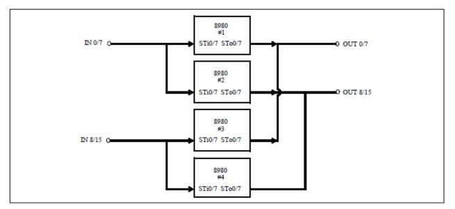
Figure 9 - Four 8980s Arranged in a Non-Blocking 16 x 16 Configuration
