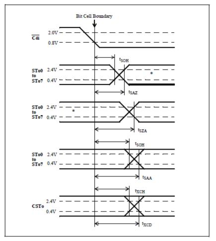
Figure 14 - Serial Outputs and External Control
