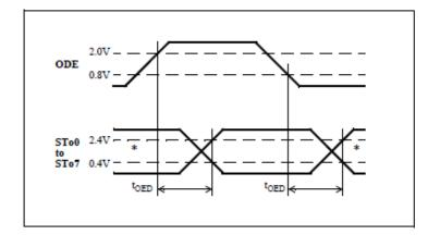
Figure 15 - Output Driver Enable
