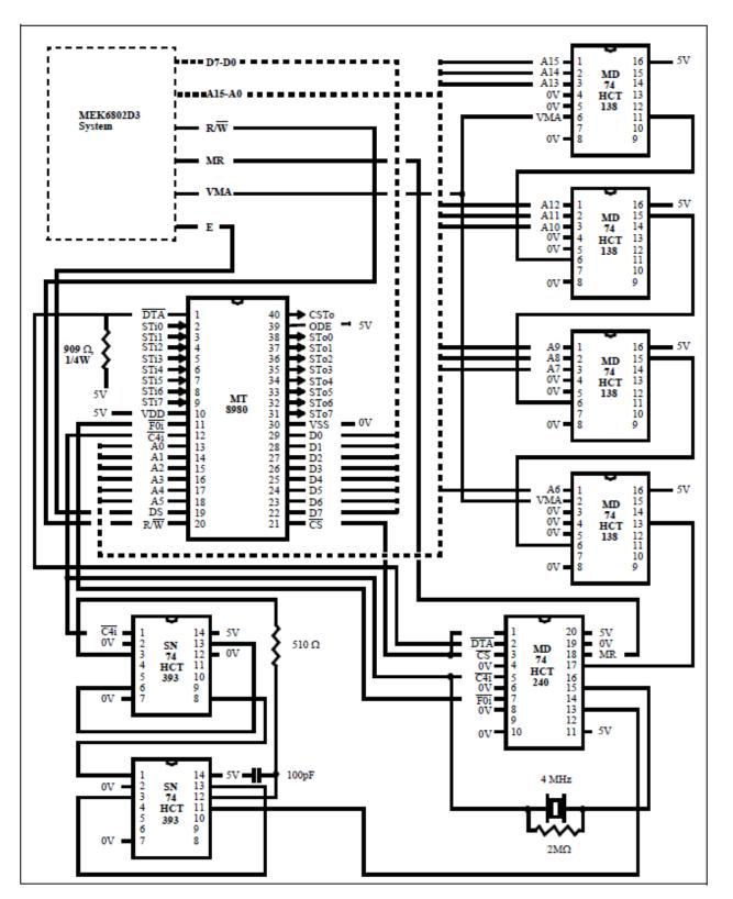
Figure 10 - Application Circuit with 6802
