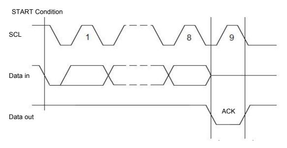
Figure 4: Timing diagram for output ACKNOWLEDGE
