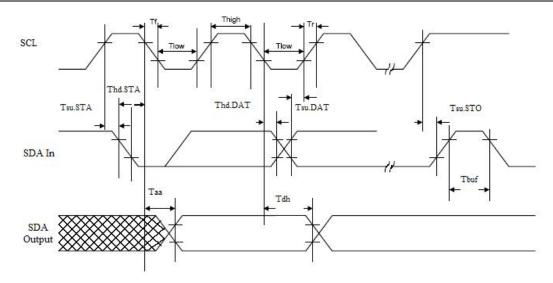
Figure 10: SCL and SDA Bus Timing
