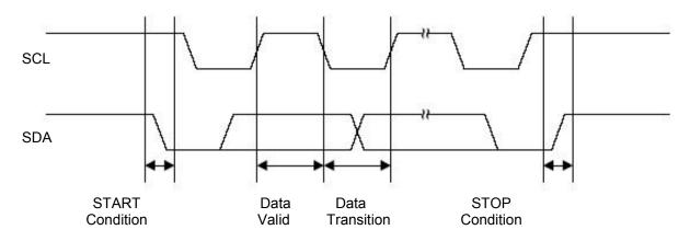
Figure 3: Timing diagram for START and STOP conditions
