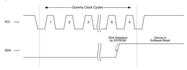
In the event that the device is still non-responsive or remains active on the SDA bus, a power cycle must be used to reset the device (see Power-Up Requirements and Reset Behavior).
