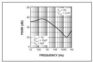
**FIGURE 2-1:** Power Supply Rejection Ratio.
