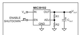
FIGURE 4-2: Adjustable Regulator with Resistors.
