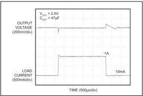
FIGURE 2-23: Load Transient Response.
