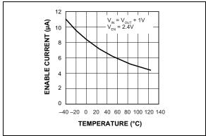
FIGURE 2-20: Enable Current vs. Temperature.
