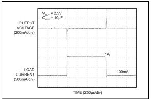
FIGURE 2-22: Load Transient Response.
