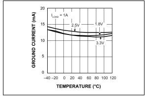
**FIGURE 2-16:** Ground Current vs. Temperature.
