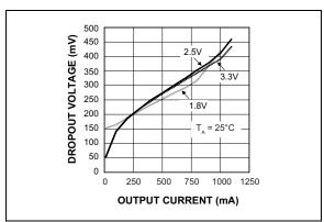
**FIGURE 2-5:** Dropout Voltage vs. Output Current.
