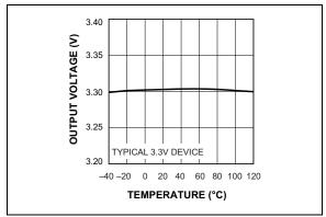
**FIGURE 2-17:** Output Voltage vs. Temperature.
