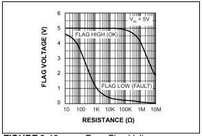
**FIGURE 2-19:** Error Flag Voltage vs. Pull-Up Resistor Value.
