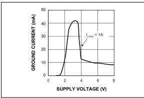
**FIGURE 2-13:** Ground Current vs. Supply Voltage (3.3V).
