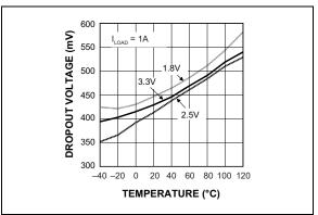
FIGURE 2-6: Dropout Voltage vs. Temperature.
