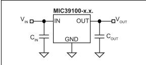
FIGURE 4-1: Capacitor Requirements.
