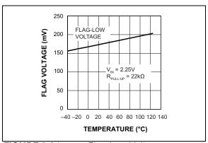
FIGURE 2-21: Flag-Low Voltage vs. Temperature.
