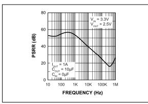
**FIGURE 2-3:** Power Supply Rejection Ratio.
