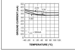
**FIGURE 2-15:** Ground Current vs. Temperature.
