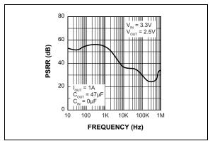
**FIGURE 2-4:** Power Supply Rejection Ratio.
