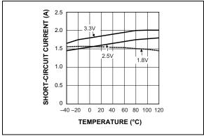
FIGURE 2-18: Short-Circuit vs. Temperature.
