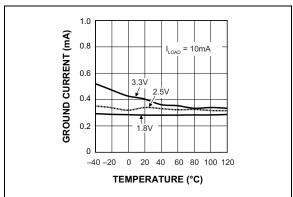
**FIGURE 2-14:** Ground Current vs. Temperature.
