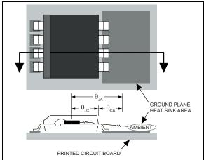
FIGURE 4-3: Thermal Resistance.
