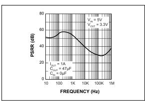
**FIGURE 2-2:** Power Supply Rejection Ratio.
