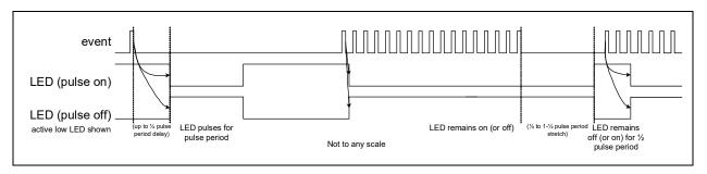
The blink / pulse stretch rate can be configured, as detailed in Section 4.12.3.1.3, "Rate of LED Blink or Pulse-Stretch".
