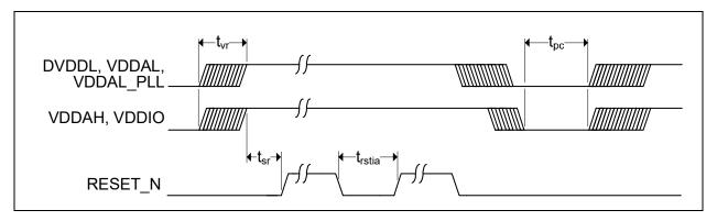
The recommended power-up sequence is to have the transceiver (AVDDH) and digital I/O (DVDDH) voltages power up before the 1.2V core (DVDDL, AVDDL\_PLL) voltage. If the 1.2V core must power up first, the maximum lead time for the 1.2V core voltage with respect to the transceiver and digital I/O voltages should be 200  $\mu$ s.
