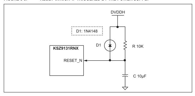
Figure 6-9 illustrates the reset circuit for applications where reset is driven by another device (for example, the CPU or an FPGA). At power-on-reset, R, C, and D1 provide the monotonic rise time to reset the KSZ9131RNX device. The RST OUT N from the CPU/FPGA provides the warm reset after power-up.
