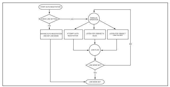
For 1000BASE-T mode, auto-negotiation is required and always used to establish a link. During 1000BASE-T auto-negotiation, the master and slave configuration is first resolved between link partners. Then the link is established with the highest common capabilities between link partners.
