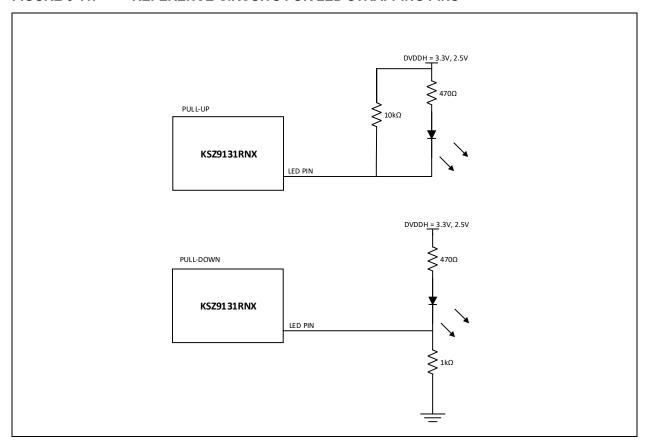
For 1.8V DVDDH, LED indication support requires voltage level shifters between LED[2:1] pins and LED indicator diodes to ensure the multiplexed PHYAD[1:0] strapping pins are latched in high/low correctly. If LED indicator diodes are not implemented, the PHYAD[1:0] strapping pins just need 10 k $\Omega$  pull-up to 1.8V DVDDH for a value of 1, and 1.0 k $\Omega$  pull-down to ground for a value of 0.
