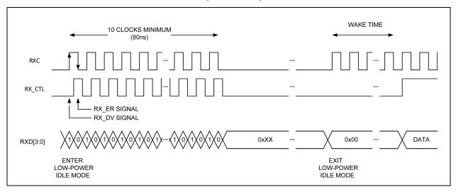
RGMII 100 Mbps reception from PHY-to-MAC uses both rising and falling edges of the RXC clock. The KSZ9131RNX uses the RX\_CTL pin to clock out the RX\_DV signal on the rising edge and the RX\_ER signal on the falling edge. It also uses the RXD[3:0] pins to clock out the RX data Bits [3:0] on the rising edge.
