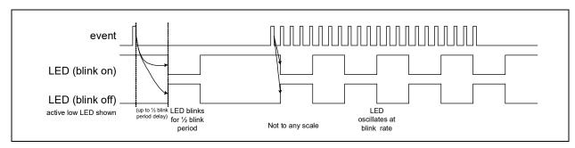
Pulse-stretch ensures that an LED is asserted and de-asserted for a specific period of time when activity is either present or not present.
