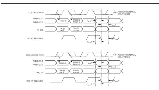
FIGURE 4-7: RGMII V2.0 SPEC (MULTIPLEXING AND TIMING DIAGRAM - ORIGINAL RGMII (V2.0) WITH INTERNAL DELAY
