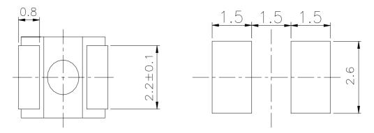
Note: The tolerances unless mentioned is ±0.1mm ;Unit = mm
