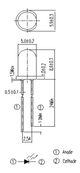
Note: Tolerances unless dimensions ±0.25mm
