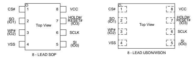
Table 1. Pin Description for SOP8/DIP8/USON8/WSON8 Package
