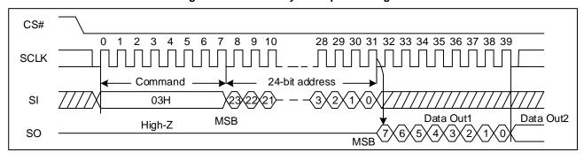
Figure 8. Read Data Bytes Sequence Diagram
