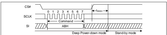
Figure 33. Release Power-Down Sequence Diagram
