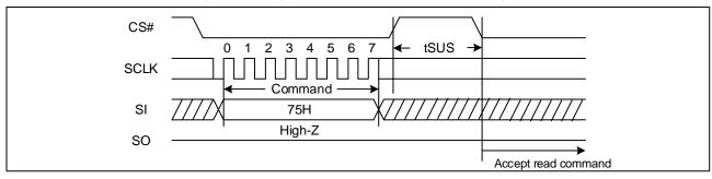
Figure 30. Program/Erase Suspend Sequence Diagram
