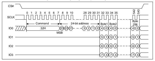
Figure 18. Quad Page Program Sequence Diagram
