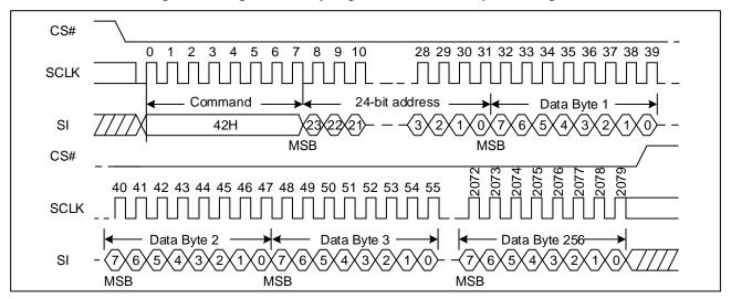
Figure 27. Program Security Registers command Sequence Diagram
