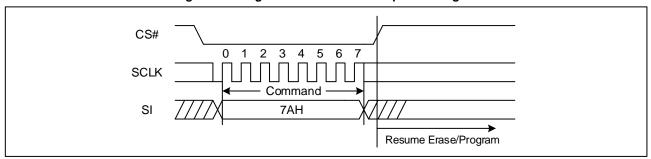
Figure 31. Program/Erase Resume Sequence Diagram
