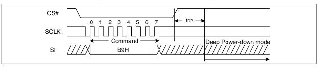
Figure 32. Deep Power-Down Sequence Diagram
