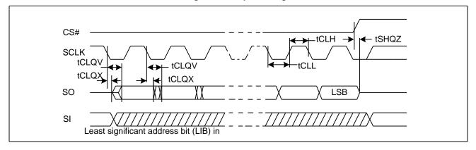
Figure 41. Resume to Suspend Timing Diagram
