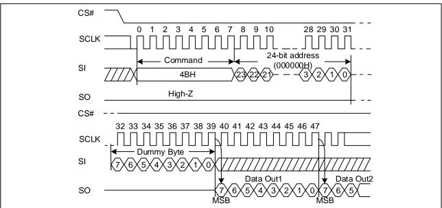
Figure 25. Read Unique ID Sequence Diagram
