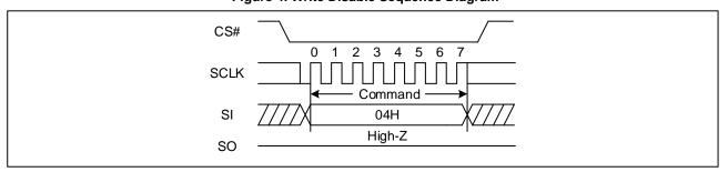
Figure 4. Write Disable Sequence Diagram
