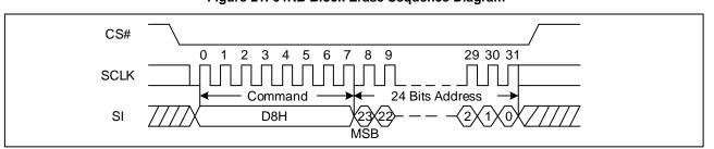
Figure 21. 64KB Block Erase Sequence Diagram
