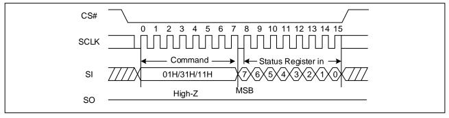
Figure 6. Write Status Register Sequence Diagram
