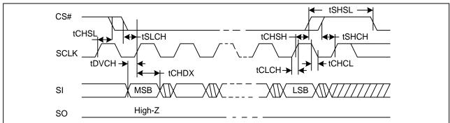
Figure 40. Output Timing
