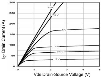
**Figure 1 Output Characteristics**
