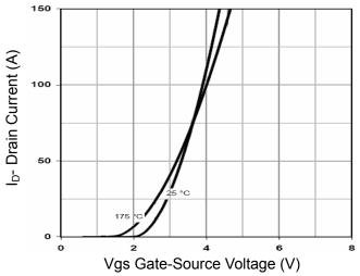
**Figure 2 Transfer Characteristics**
