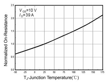
Figure 4 Rdson-JunctionTemperature
