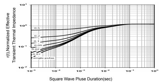
**Figure 11 Normalized Maximum Transient Thermal Impedance**
