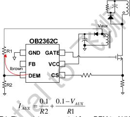
R1: The resistor connected from DEM to AUX. R2: The resistor connected from DEM to ground. When system starts up, if  $I_{AUX} < I_{brown_in}$ , Brown-in auto-recovery protection is triggered after 2 Gate cycles debounce. When the system enters the normal operation mode, if  $I_{AUX} < I_{brown_out}$ , Brownout auto-recovery protection is triggered after 29ms debounce.
