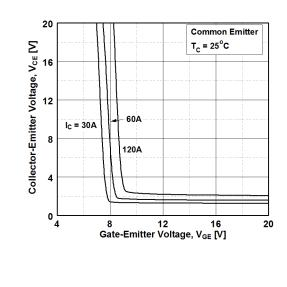
**Figure 2. Typical Output Characteristics**
