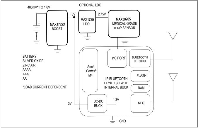
Figure 7. MAX1722x/MAX30205 Temperature Sensor Wearable Solution
