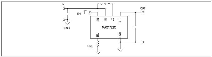
Figure 6. Single R<sub>SEL</sub> Resistor Sets the Output Voltage
