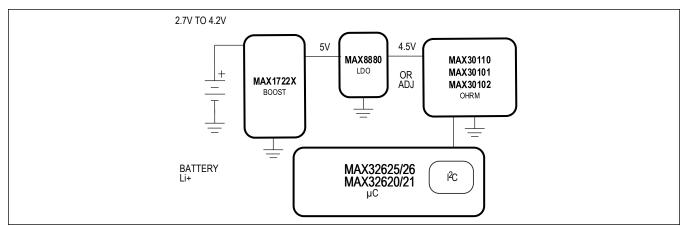
Figure 9. MAX1722x/MAX30110/MAX30101/MAX30102 Optical Heart Rate Monitor (OHRM) Sensor Wearable Solution for Secondary Cells
