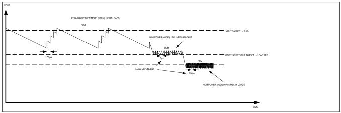
Figure 4. ULPM, LPM, and HPM Waveforms (Part 1)
