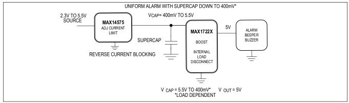
Figure 11. MAX1722x/MAX14575 Solution for Alarm Beeper Buzzers
