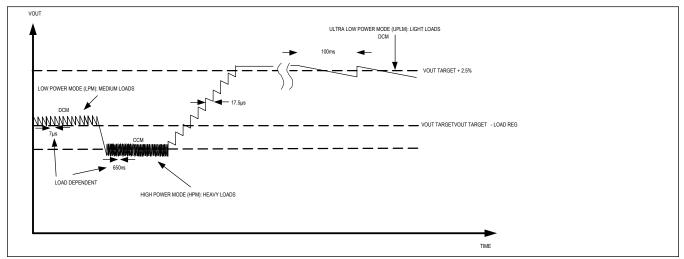
Figure 5. ULPM, LPM, and HPM Waveforms (Part 2)
