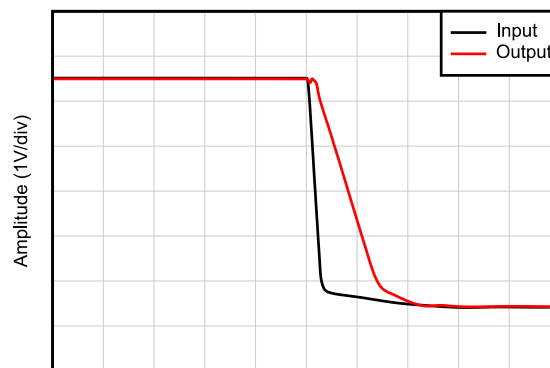
Figure 6-32. Small-Signal Step Response, Falling
