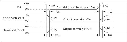
Figure 9. Receiver Enable and Disable Times
