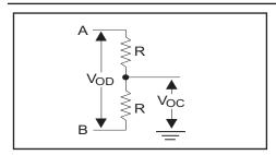
Figure 2. Driver DC Test Load Circuit
