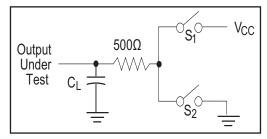
Figure 5. Driver Timing Test Load #2 Circuit
