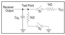
Figure 3. Receiver Timing Test Load Circuit
