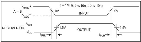
Figure 8. Receiver Propagation Delays
