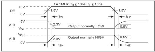
Figure 7. Driver Enable and Disable Times
