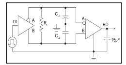
Figure 4. RS-485 Driver/Receiver Timing Test
