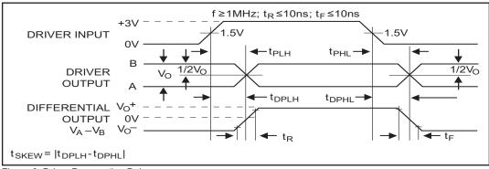
Figure 6. Driver Propagation Delays
