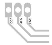
Figure 21. TO-92 LP Package Recommended Layout
