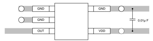
Figure 20. SC70 Package Recommended Layout
