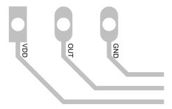
Figure 22. TO-92 LPM Package Recommended Layout
