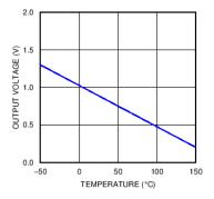
Figure 14. Analog Output Transfer Function
