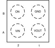
Figure 5-1. YFP Package 4-Pin WSON Laser Marking View
