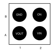
Figure 5-2. YFP Package 4-Pin WSON Bump View
