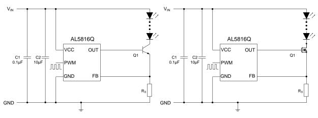
Figure 1. Typical Application Circuit Using BJT and MOSFET
