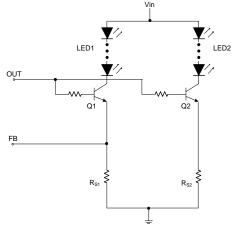
Figure 2. Two LED Strings in Parallel
