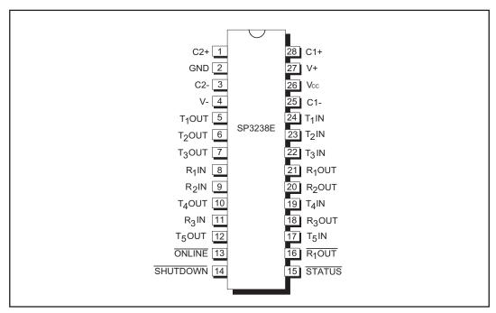
Figure 4. SP3238E Pinout Configuration
