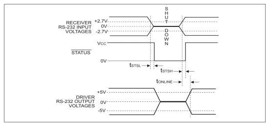
Figure 16. AUTO ON-LINE® Timing Waveforms
