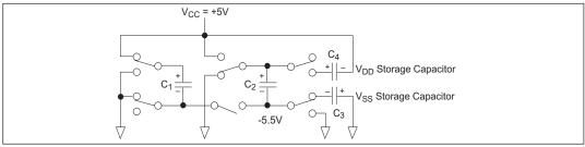
Figure 12. Charge Pump — Phase 2
