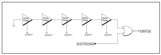
Figure 18. Stage II of AUTO ON-LINE® Circuitry
