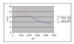
Figure 2. Slew Rate VS. Load Capacitance
