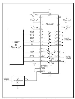
Figure 6. Interface Circuitry Controlled by Microprocessor Supervisory Circuit
