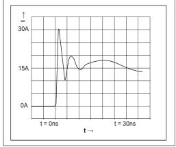
Figure 21. ESD Test Waveform for IEC61000-4-2
