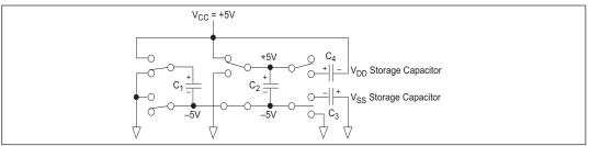
Figure 11. Charge Pump — Phase 1
