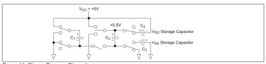
Figure 14. Charge Pump — Phase 4
