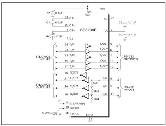
Figure 5. SP3238E Typical Operating Circuit
