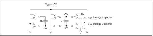
Figure 13. Charge Pump — Phase 3
