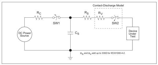
Figure 20. ESD Test Circuit for IEC61000-4-2
