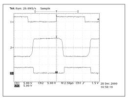
Figure 8. Loopback Test results at 120kbps (All Drivers Fully Loaded)
