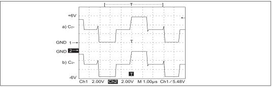
Figure 17. Charge Pump Waveforms
