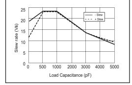
Figure 5. Slew Rate vs Load Capacitance for the SP3220EB.
