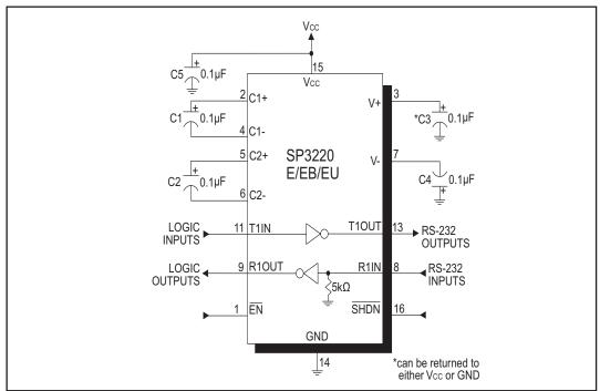
Figure 11. SP3220E/EB/EU Typical Operating Circuit
