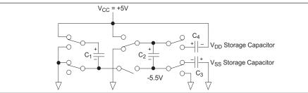
Figure 16. Charge Pump — Phase 2
