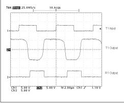
Figure 13. SP3220EB Loopback Test results at 250kbps
