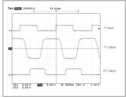
Figure 14. SP3220EU Loopback Test results at 1Mbps
