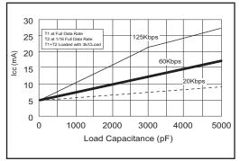
Figure 1. Icc vs Load Capacitance for the SP3220EB.
