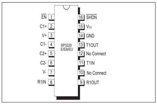
Figure 10. Pinout Configurations for the SP3220E/EB/EU
