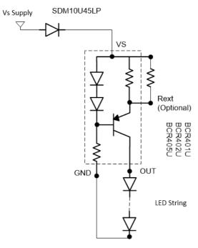
Figure 9. Application Circuit for LED Driver with Reverse Polarity Protection
