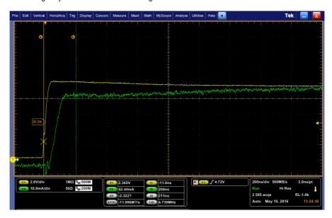
Figure 5. Turn On Time of BCR401/2/5 (PWM Method Shown in Figure 3b)
