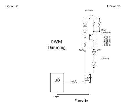
Figure 3a, 3b & 3c. Application Circuits for LED Driver with PWM Dimming Functionality
