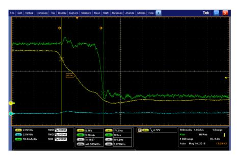
Figure 7. Turn Off Time of BCR401/2/5 While Switching the Power Path as Shown in Figure 3c  $\,$
