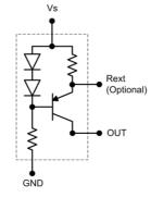
Internal Device Schematic
