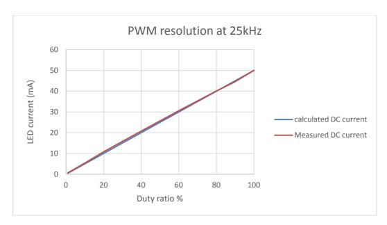
Figure 8. PWM Resolution with Power Path Switching (Refer to Figure 3c)
