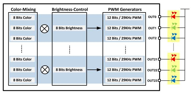
Figure 9. PWM Control Scheme for Each Channel
