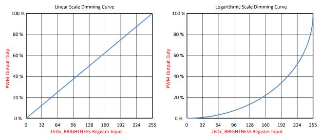
Figure 11. Logarithmic vs Linear Dimming Curve
