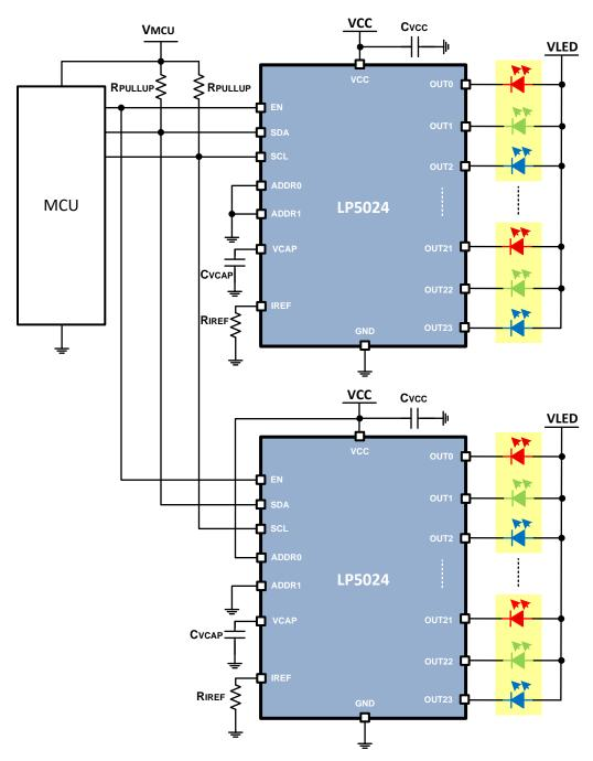
Figure 61. Driving Dual LP5024 Application Example
