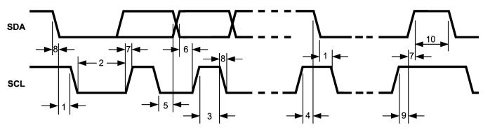
Figure 1. I<sup>2</sup>C Timing Parameters
