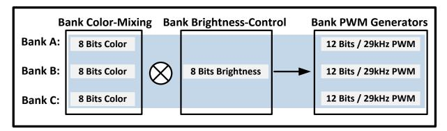
Figure 13. Bank PWM Control Scheme
