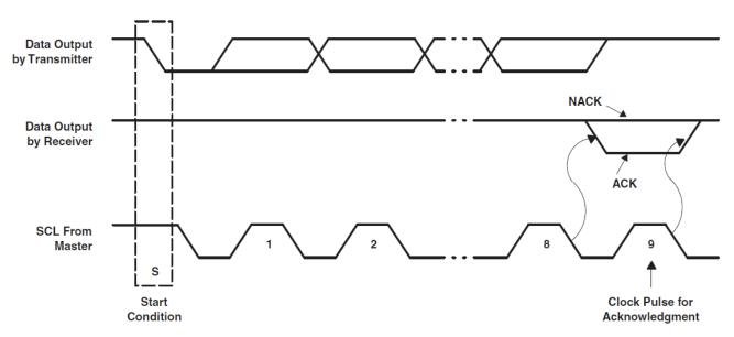
Figure 18. Acknowledge and Not Acknowledge on I<sup>2</sup>C Bus
