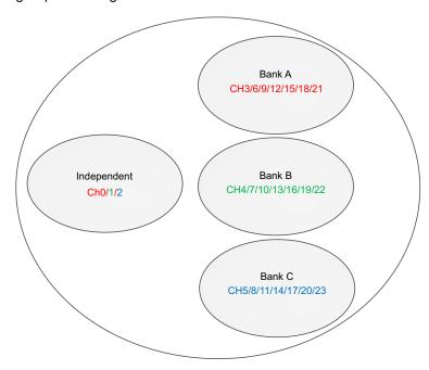
Figure 14. Bank PWM Control Example
