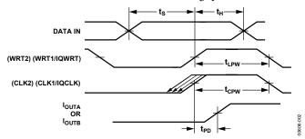
Figure 2. Timing for Dual and Interleaved Modes
