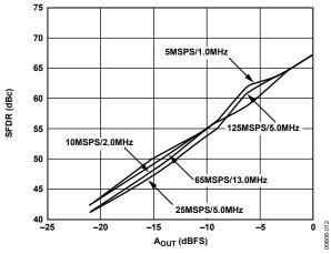
Figure 11. Single-Tone SFDR vs.  $A_{OUT} @ f_{OUT} = f_{CLK}/5$
