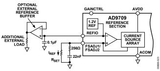
Figure 23. Internal Reference Configuration
