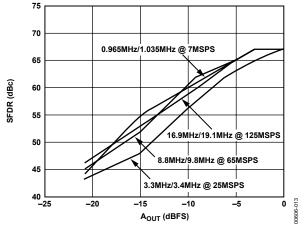
Figure 12. Dual-Tone SFDR vs. Aout @  $f_{OUT} = f_{CLK}/7$
