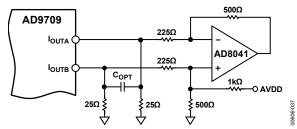
Figure 38. Single-Supply DC Differential Coupled Circuit
