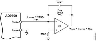
Figure 40. Unipolar Buffered Voltage Output
