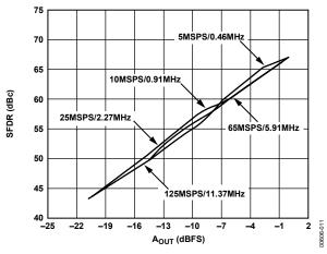
Figure 10. Single-Tone SFDR vs.  $A_{OUT} @ f_{OUT} = f_{CLK}/11$
