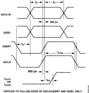
Figure 28. 5 V or 3.3 V Interleaved Mode Timing
