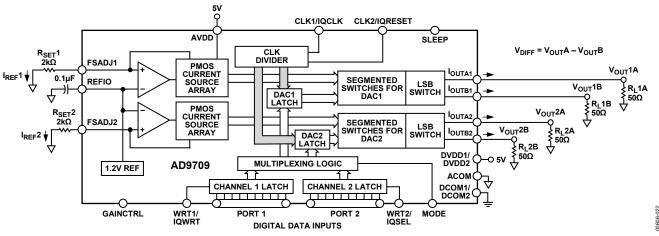
Figure 22. Simplified Block Diagram
