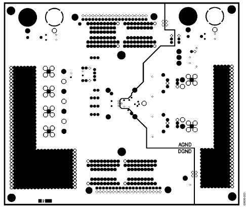
Figure 52. Layer 2, Ground Plane
