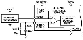
Figure 24. External Reference Configuration
