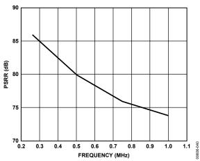
Figure 41. AVDD Power Supply Rejection Ratio vs. Frequency
