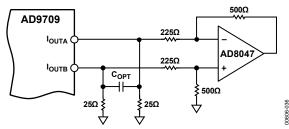
Figure 37. DC Differential Coupling Using an Op Amp
