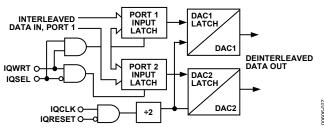
Figure 25. Latch Structure in Interleaved Mode
