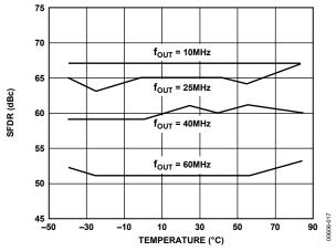
Figure 16. SFDR vs. Temperature @  $f_{CLK} = 125$  MSPS, 0 dBFS
