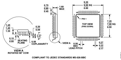
Figure 55. 48-Lead Low Profile Quad Flat Package [LQFP] (ST-48) Dimensions shown in millimeters
