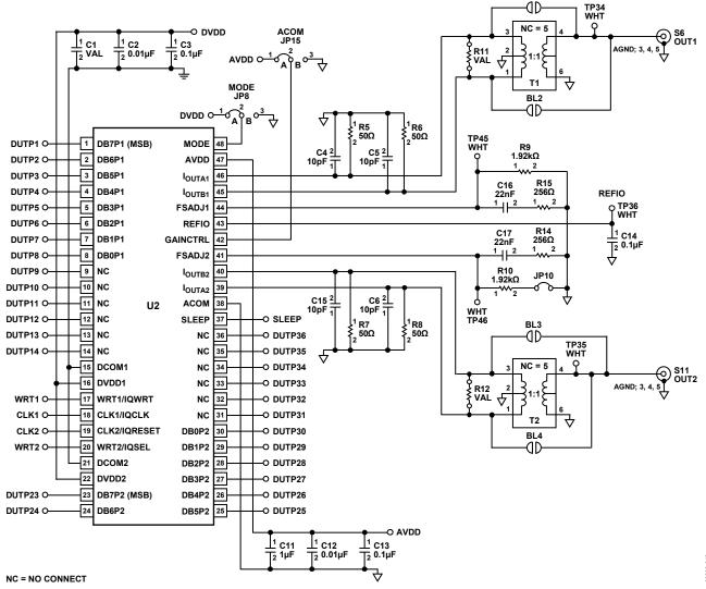
Figure 48. AD9709 and Output Signal Conditioning
