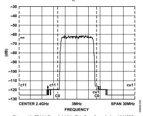
Figure 45. CDMA Signal, 8 MHz Chip Rate Sampled at 65 MSPS, Recreated at 2.4 GHz, Adjacent Channel Power > 54 dB
