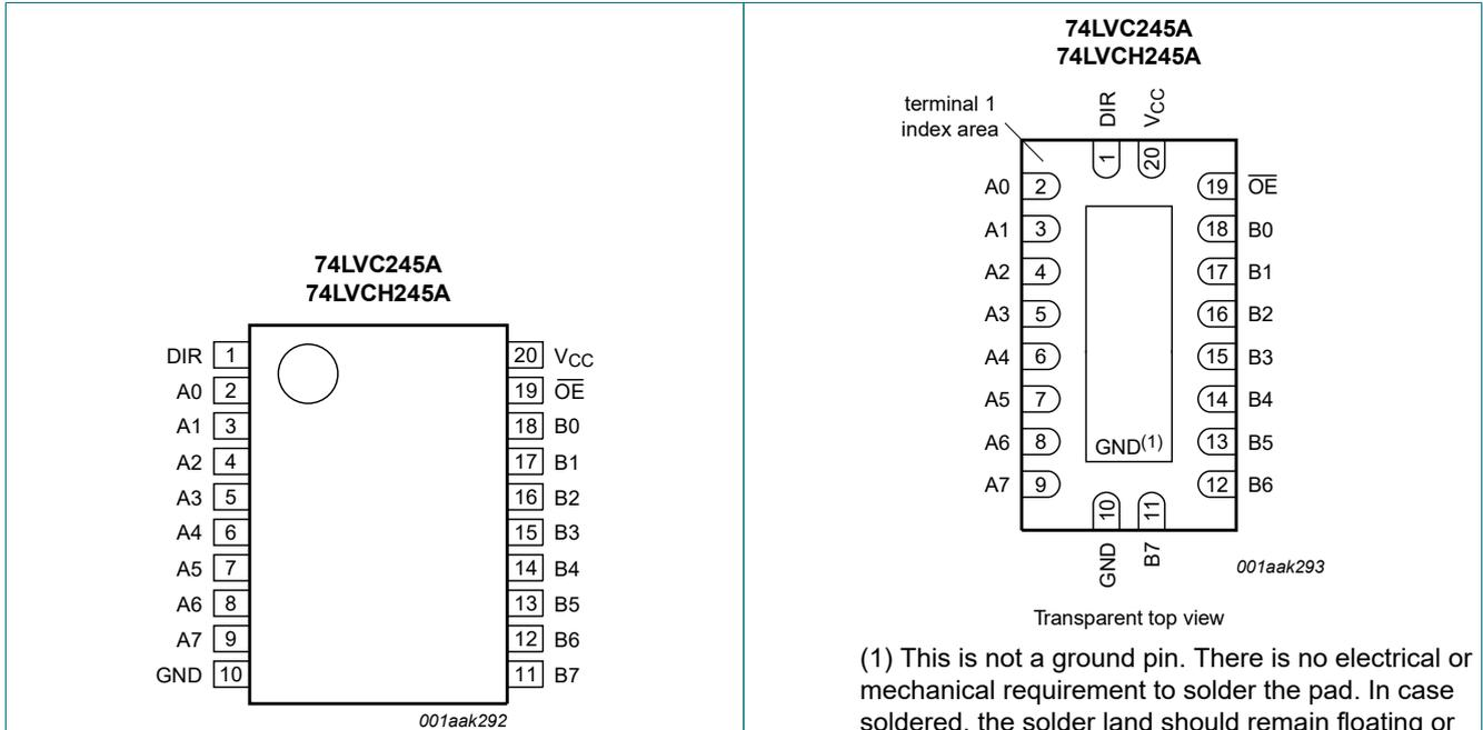
Fig. 3. Pin configuration SOT163-1 (SO20) and SOT360-1 (TSSOP20)
