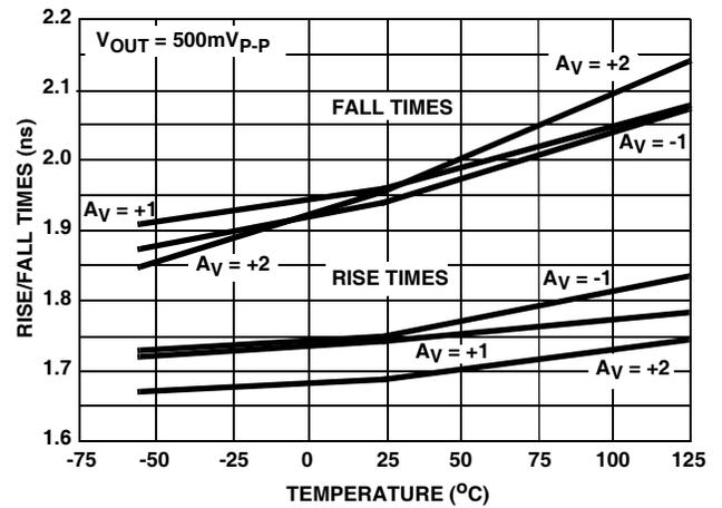
FIGURE 35. RISE AND FALL TIMES vs TEMPERATURE
