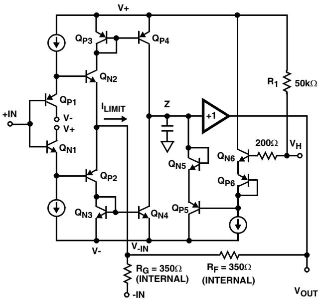
FIGURE 3. HFA1115 SIMPLIFIED V<sub>H</sub> LIMIT CIRCUITRY
