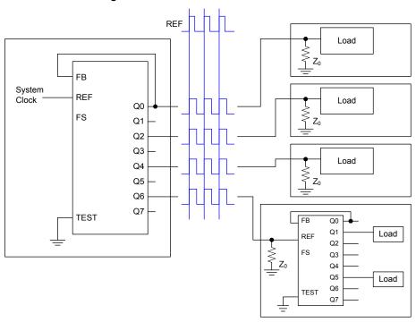
Figure 5. Board-to-Board Clock Distribution
