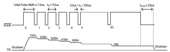
Figure 2. UM1663S pulse dimming
