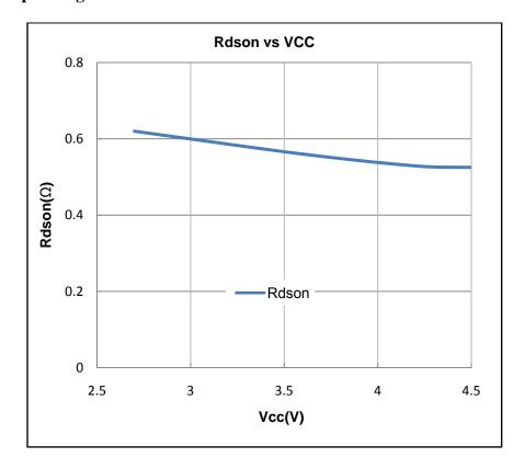
Internal Power NMOS Rds(on) Vs VCC Curve
