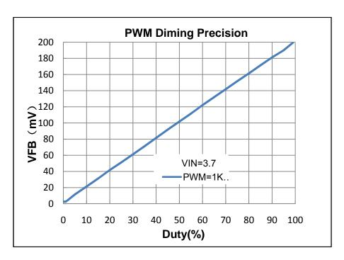
PWM Dimming Pulse vs  $V_{FB}$  Voltage Curve
