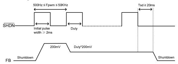
Figure 1. UM1663S PWM dimming
