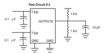
For parameter t<sub>8</sub> (output slew rate) on -1H devices
