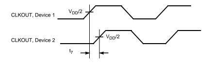
Figure 9. Stop Time between Change in Input Reference Frequency
