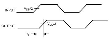
Figure 8. Device-Device Skew
