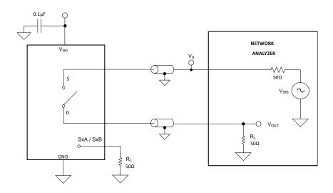
Figure 22. Off Isolation Measurement Setup
