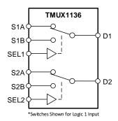
Figure 25. TMUX1136 Functional Block Diagram
