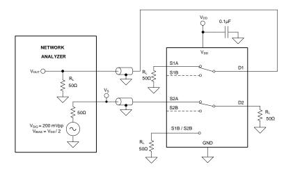
Figure 23. Crosstalk Measurement Setup
