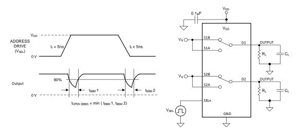
Figure 20. Break-Before-Make Delay Measurement Setup
