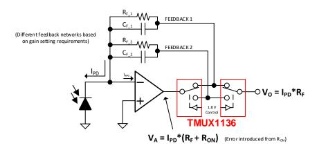
Figure 29. Transimpedance Amplifier Feedback Switching
