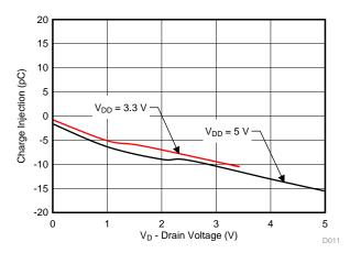
Figure 28. Charge Injection vs Drain Voltage
