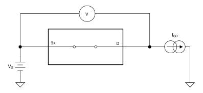
Figure 16. On-Resistance Measurement Setup
