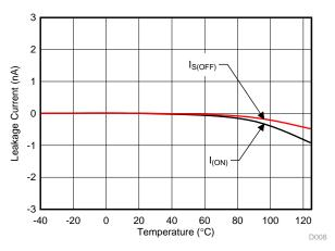
Figure 26. Leakage Current vs Temperature
