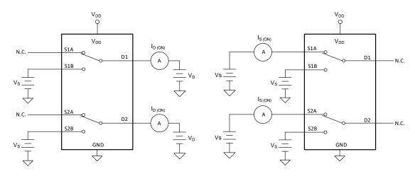
Figure 18. On-Leakage Measurement Setup
