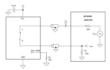
Figure 24. Bandwidth Measurement Setup
