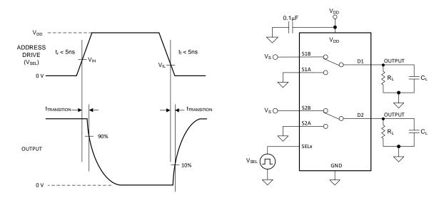
Figure 19. Transition-Time Measurement Setup
