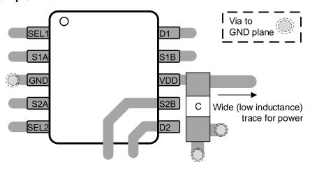
Figure 32. TMUX1136 Layout Example
