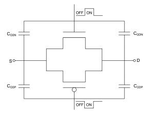
Figure 27. Transmission Gate Topology
