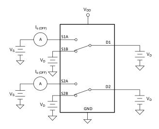
Figure 17. Off-Leakage Measurement Setup
