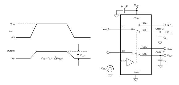
Figure 21. Charge-Injection Measurement Setup
