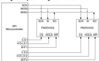
Figure 3. System Configuration with SPI Port
