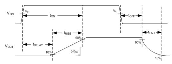
Figure 32. Timing Waveforms
