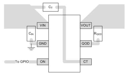
Figure 38. Recommended Board Layout
