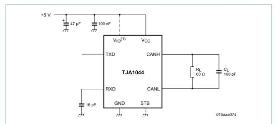
(1) The  $V_{IO}$  pin is internally connected to pin  $V_{CC}$  in the non- $V_{IO}$  product variants TJA1044(G)T(K).
