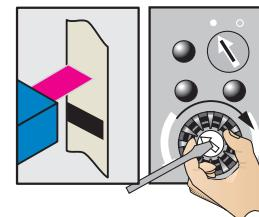
Turn the potentiometer forward again by half the number of turns to ensure that the switching threshold is optimally set.
