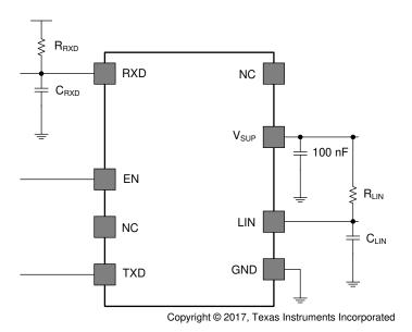
Figure 25. Test Circuit for AC Characteristics
