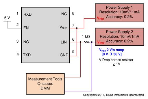
Figure 16. Test Circuit for  $I_{BUS\ NO\ GND}$  Loss of GND
