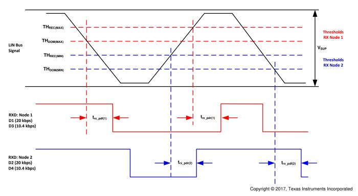
Figure 21. Propagation Delay
