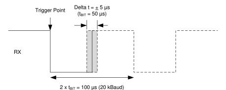
Figure 9. RX Response: Operating Voltage Range
