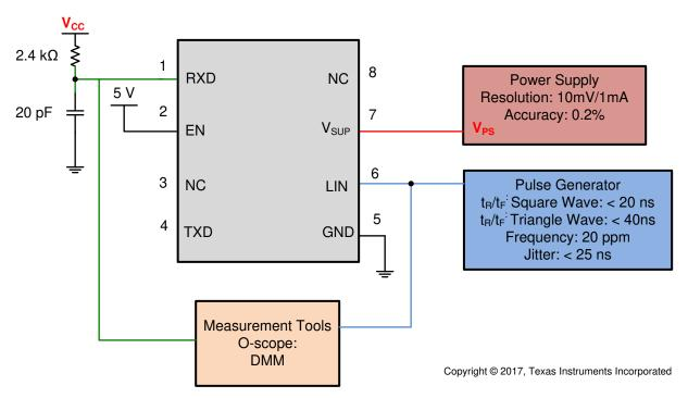
Figure 20. Propagation Delay Test Circuit; Param 31, 32
