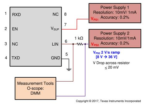
Figure 15. Test Circuit for I<sub>BUS\_PAS\_rec</sub> Param 14
