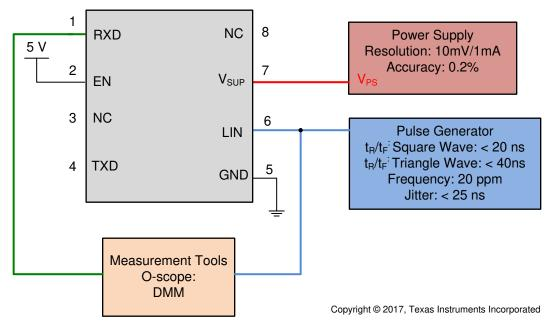
Figure 11. LIN Receiver Test with RX access Param 17, 18, 19, 20
