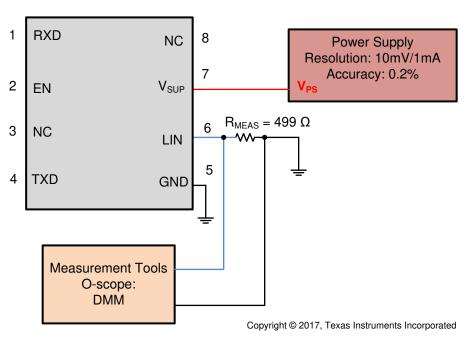
Figure 14. Test Circuit for I<sub>BUS PAS dom</sub>; TXD = Recessive State V<sub>BUS</sub> = 0 V, Param 13
