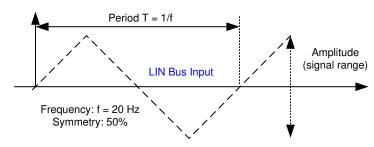
Figure 10. LIN Bus Input Signal
