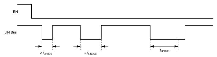
Figure 27. No Bus Fault: Entering Sleep Mode with Bus Recessive Condition and Wakeup
