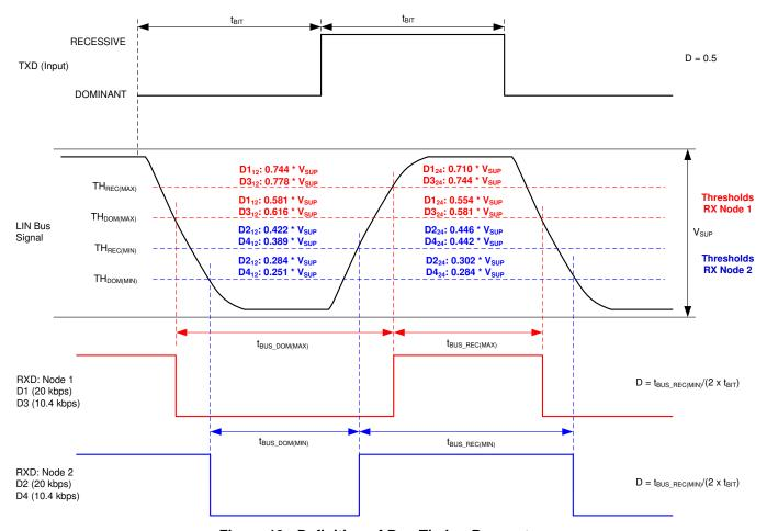
Figure 19. Definition of Bus Timing Parameters
