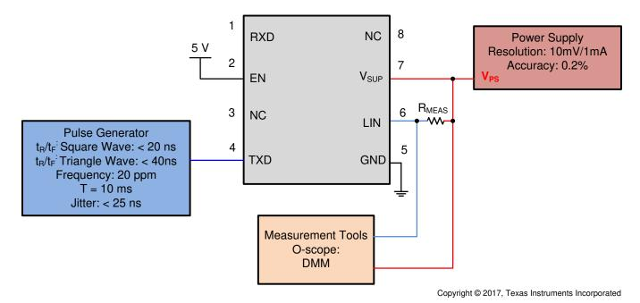
Figure 13. Test Circuit for I<sub>BUS LIM</sub> at Dominant State (Driver on) Param 12
