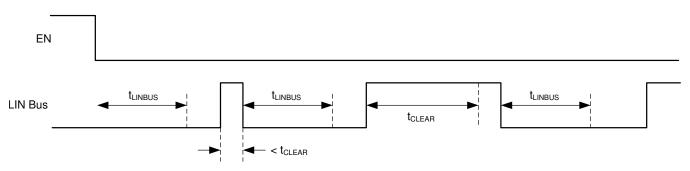
Figure 28. Bus Fault: Entering Sleep Mode with Bus Stuck Dominant Fault, Clearing, and Wakeup
