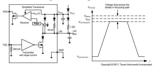
Figure 26. Master Node Configuration with Voltage Levels
