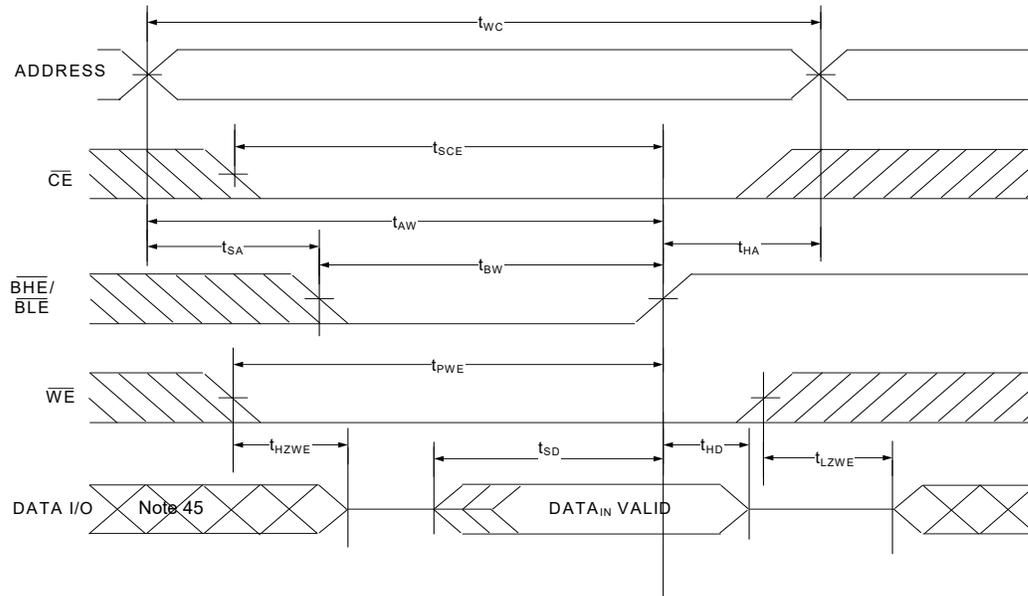
Figure 14. Write Cycle No. 5 ( $\overline{\text{WE}}$  Controlled) [42, 43, 44]
