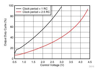
Figure 21. Pulse-Width-Modulation vs Control Voltage Clock Duty Cycle 98%, V<sub>DD</sub> = 5 V
