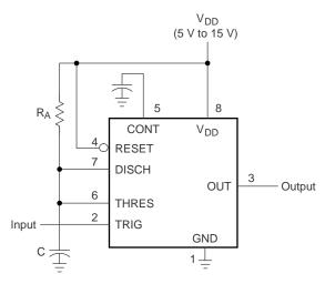
Figure 9. Circuit for Monostable Operation
