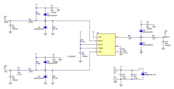
Figure 27. ESD Test Schematic
