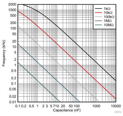
Figure 15. Free-Running Frequency vs Timing Capacitance Resistance =  $R_A + 2 \times R_B$
