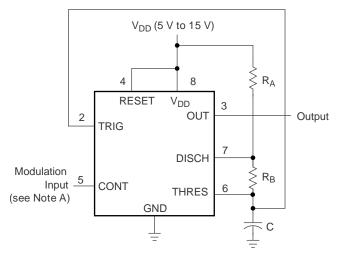
A. The modulating signal can be direct or capacitively coupled to CONT. For direct coupling, consider the effects of modulation source voltage and impedance on the bias of the timer.
