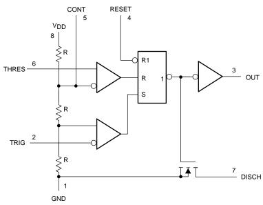
Pin numbers are for all packages except the PW and FK package. RESET can override TRIG, which can override THRES (when CONT pin is  $2/3 \, V_{DD}$ ).
