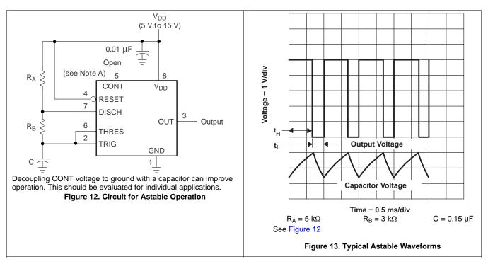
Figure 13 shows typical waveforms generated during a stable operation. The output high-level duration  $t_H$  and low-level duration  $t_I$  for frequencies below 100 kHz can be calculated as follows:
