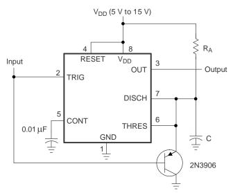
Figure 18. Circuit for Missing-Pulse Detector
