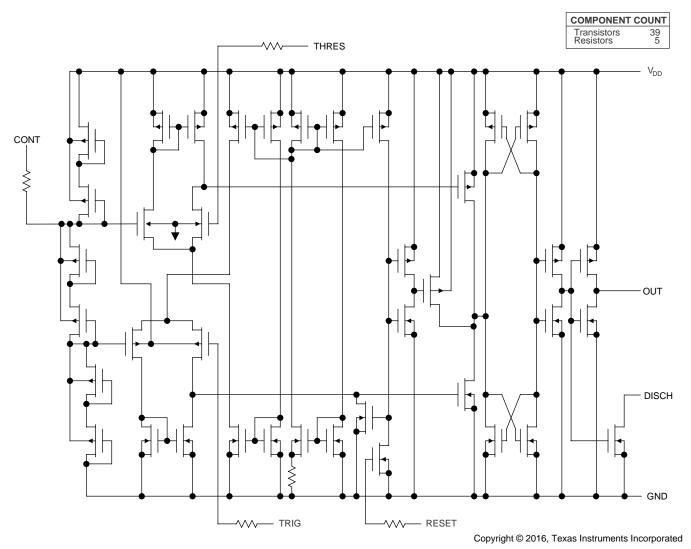
Figure 17. Equivalent Schematic
