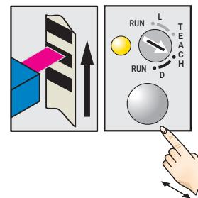
Release the teach-in button. Yellow LED will illuminate, when emitted light is on the mark.
