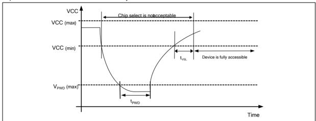
Figure 58c. Power Cycle Requirement
