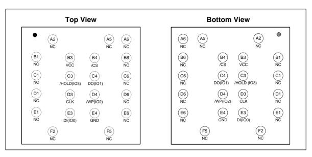
Figure 1e. W25Q128JW Ball Assignments, 21-ball WLCSP (Package Code BY)
