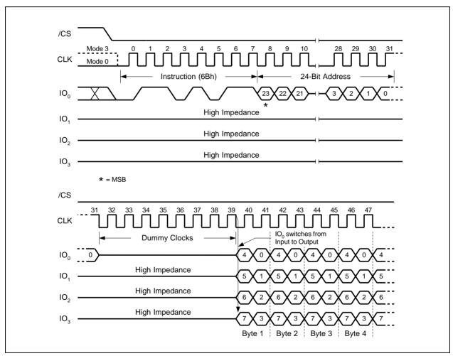
Figure 20. Fast Read Quad Output Instruction
