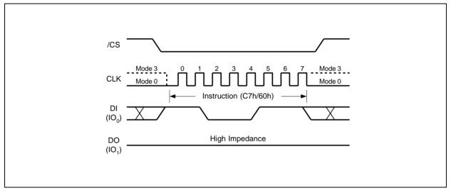
Figure 34. Chip Erase Instruction Sequence Diagram
