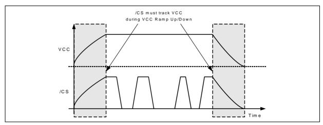
Figure 58b. Power-up, Power-Down Requirement
