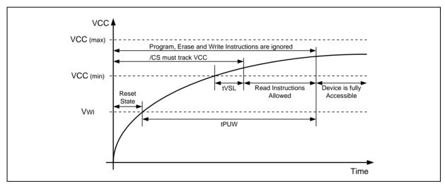
Figure 58a. Power-up Timing and Voltage Levels
