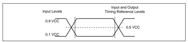
Figure 59. AC Measurement I/O Waveform
