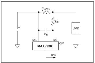
Figure 1. Differential Input Filter
