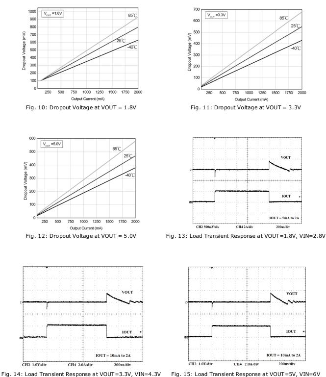
Fig. 15: Load Transient Response at VOUT=5V, VIN=6V
