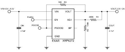
Fig. 23: 5V to 3.3V / 2A
