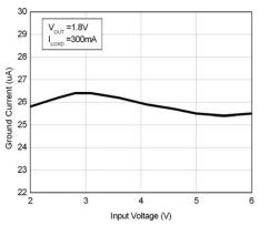
Fig. 6: GND Current vs. VIN at VOUT=1.8V, 300mA
