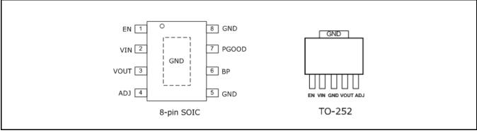
Fig. 3: XRP6272 Pin Assignment
