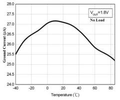
Fig. 8: GND Current vs. Temp. at VOUT=1.8V, No Load
