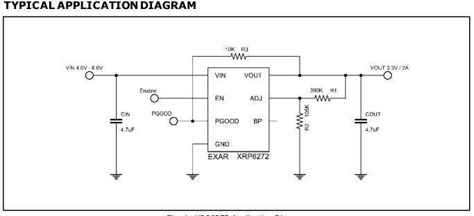
Fig. 1: XRP6272 Application Diagram
