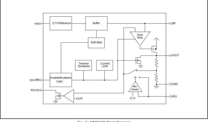
Fig. 2: XRP6272 Block Diagram
