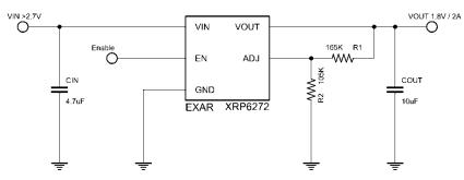
Fig. 25: 2.7V Min to 1.8V / 2A Power Supply
