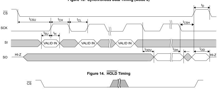
Figure 13. Synchronous Data Timing (Mode 0)
