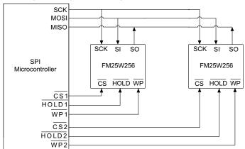
Figure 2. System Configuration with SPI port
