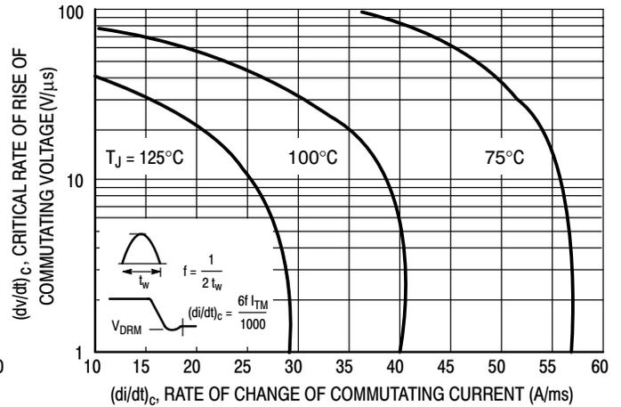
Figure 9. Critical Rate of Rise of Commutating Voltage
