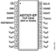
Figure 3. Pin Configuration
