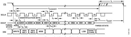
Figure 2. Serial Interface Timing Diagram
