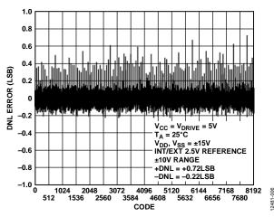
Figure 6. Typical DNL True Differential Mode
