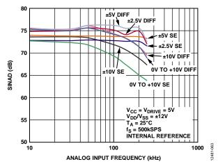
Figure 13. SINAD vs. Analog Input Frequency for Single-Ended (SE) and True Differential (Diff) Mode at 5 V V<sub>CC</sub>
