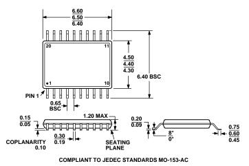
Figure 23. 20-Lead Thin Shrink Small Outline Package [TSSOP] (RU-20) Dimensions show in millimeters
