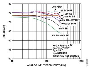
Figure 12. SINAD vs. Analog Input Frequency for Single-Ended (SE) and True Differential (Diff) Mode at 3 V V<sub>CC</sub>
