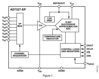
The ADC contains a 2.5 V internal reference. The AD7327-EP also allows external reference operation. If a 3 V reference is applied to the REFIN/OUT pin, the AD7327-EP can accept a true bipolar  $\pm 12$  V analog input. Minimum  $\pm 12$  V V<sub>DD</sub> and V<sub>SS</sub> supplies are required for the  $\pm 12$  V input range. The ADC has a high speed serial interface that can operate at throughput rates up to 500 kSPS.
