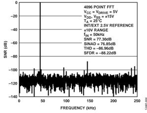
Figure 4. FFT True Differential Mode
