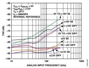
Figure 11. THD vs. Analog Input Frequency for Single-Ended (SE) and True Differential (Diff) Mode at 5 V V<sub>CC</sub>
