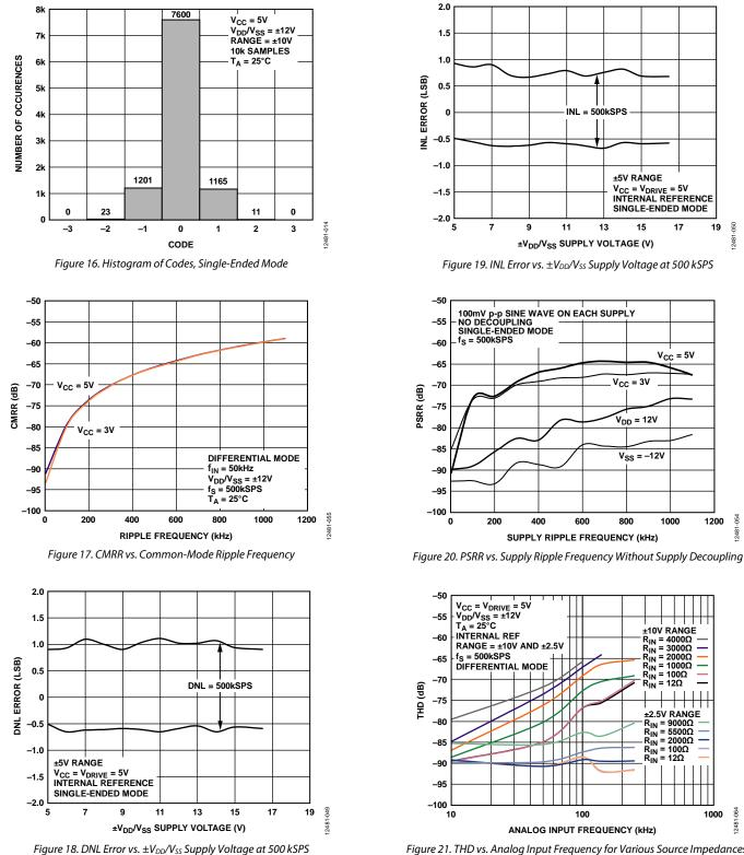
Figure 21. THD vs. Analog Input Frequency for Various Source Impedances, True Differential Mode
